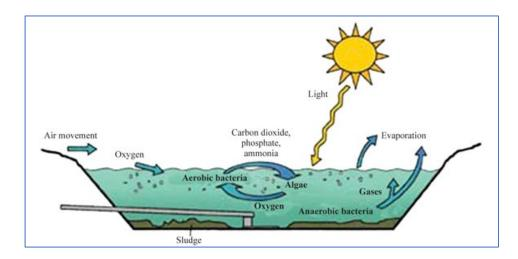
In our lagoon, untreated wastewater passes through an inlet manhole (the "main inlet") and then travels through a 700-foot pipe to the far end of the lagoon. After that, natural processes clean the wastewater as it returns to the near end, where it exits through an outlet and is channelled into the river.
